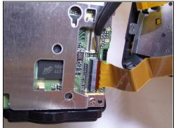
• Use needle-nose <u>tweezers</u> to gently lift the black/grey latch towards the ribbon-wire (the latch rotates upward to release and snaps down to lock).
