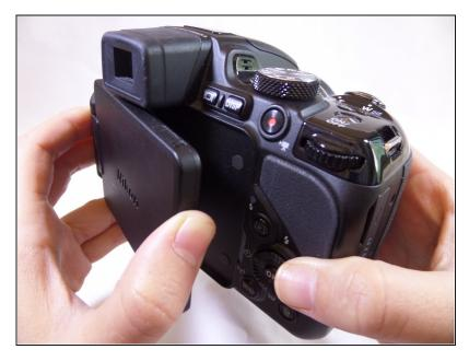
Position the back of the camera facing you and open the LCD screen to the left.
