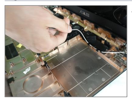
Carefully free up the black and white RF cables that are running along the laptop casing and speaker housing.
