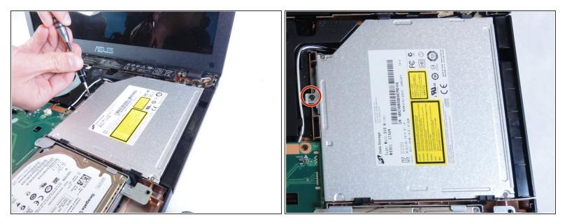
• Remove the single screw that is holding the drive in place using the Phillips #1 Screwdriver.
