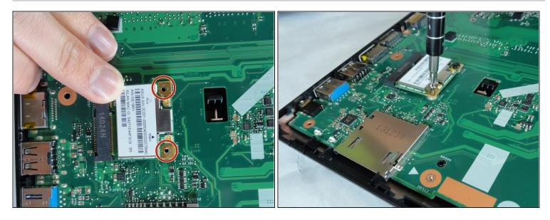
Remove the screws that are holding down the wireless network card with the Phillips #1 screwdriver.
