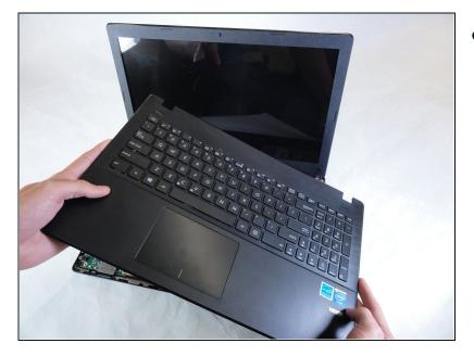
• Remove the fully disconnected keyboard module from the laptop.
