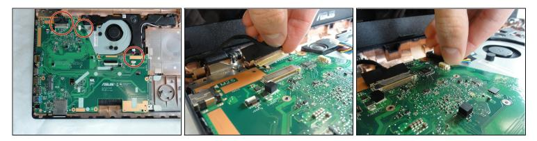
• Disconnect the three cables attached to the motherboard.
