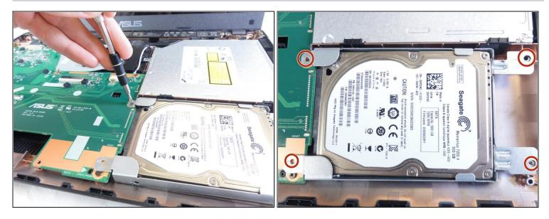
• Remove the four screws that hold the hard drive in place with the Philips #1 screwdriver.
