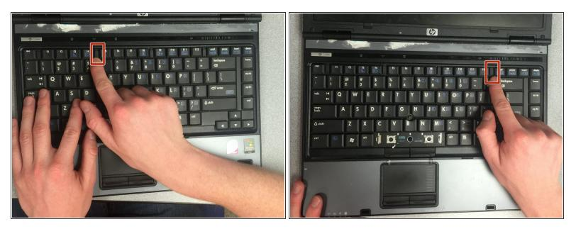
Slide the indicated tabs upward to release the keyboard.
