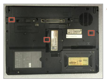
Loosen the three 1.5 cm Phillips #1 screws for the keyboard on the back of the laptop.
