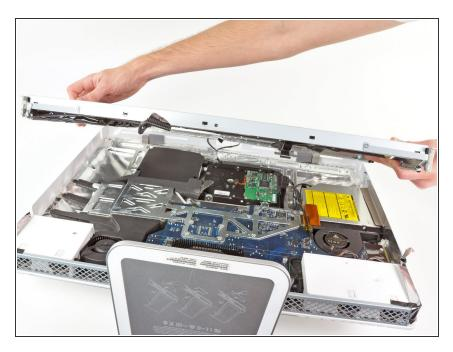
Remove the display assembly from the iMac.
