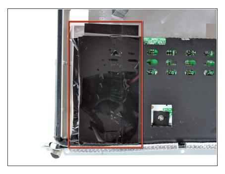
Remove the large piece of black tape covering the side of the inverter board.
