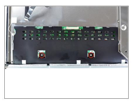
Remove the two Phillips screws securing the inverter board to the back of the LCD.
