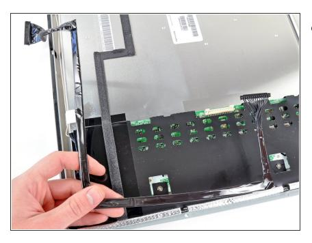
Remove the inverter cable from the LCD.
