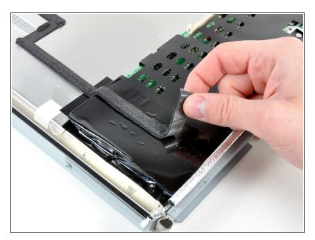
Peel the strip of foam tape off the inverter board.
