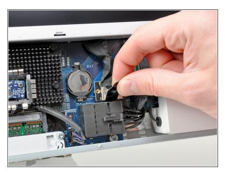
Pull the black plastic tab attached to the display data cable connector to disconnect it from the logic board.
