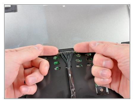
Lift the inverter cable connector straight up from its socket on the inverter board.
