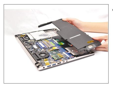
Remove the battery completely.
