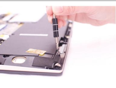
Remove the eight 3 mm Phillips #0 screws on the bottom panel.
