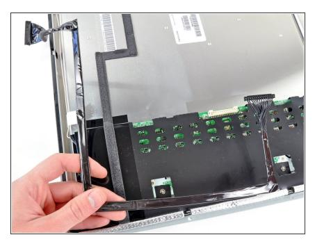
Remove the inverter cable from the LCD.
