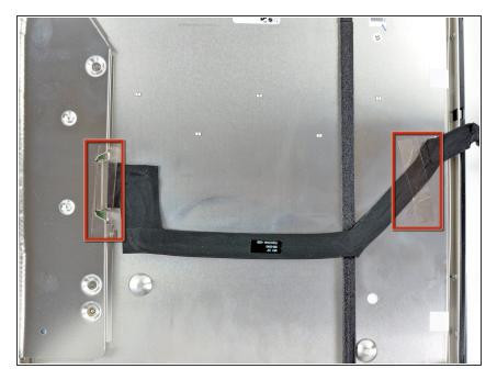
Remove the two pieces of tape securing the display data cable to the back of the display.
