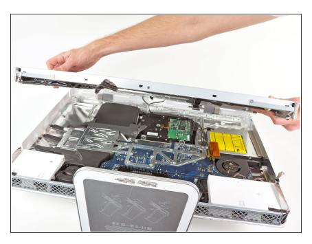
Remove the display assembly from the iMac.
