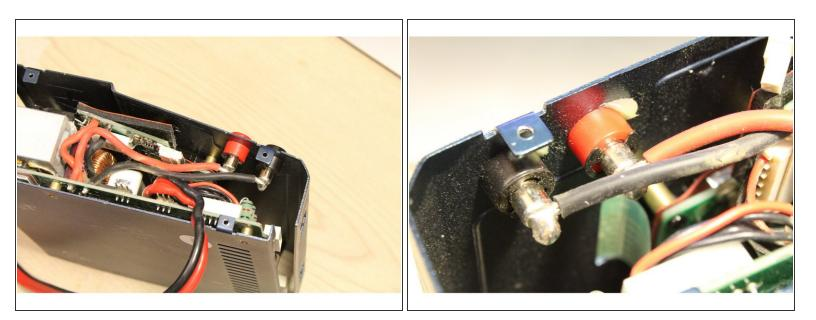
• Desolder the two wires connected to the female banana plug ports for both channel 1 and 2 (left and ride sides of the charger).
