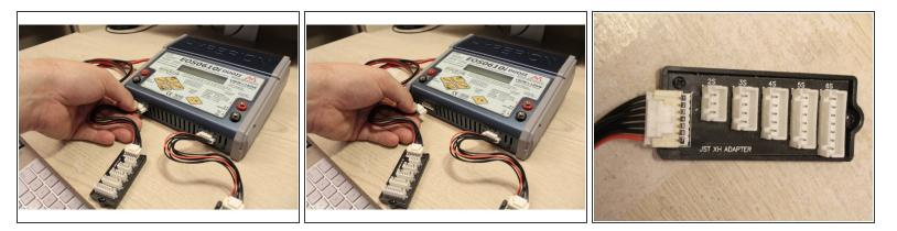
Press down on the tab located on the top of the white molex connector and firmly pull away from the charger body.
