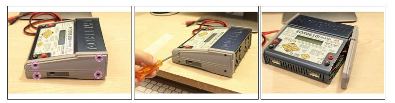
• Remove the four screws located on the right side cover of the charger.
