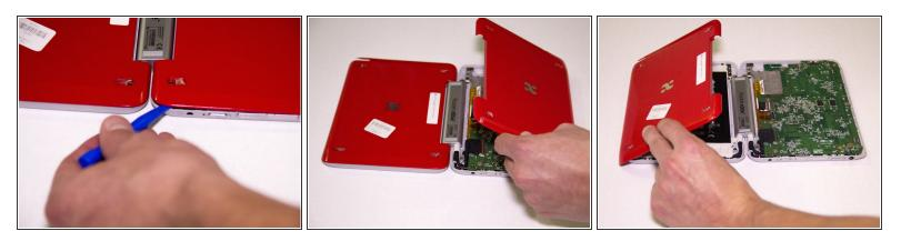
• Using the plastic opening tool, lift the back plate from both sides of your device and remove them.
