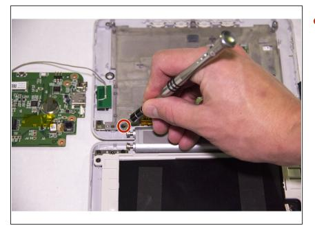
Using your J0 Phillips head screwdriver, remove the one 5 mm screw holding the gray plastic ereader screen backing into place.
