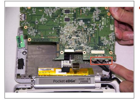
Lift the outer edge of the motherboard up. Carefully disconnect the 3 connections on bottom of the motherboard by pulling gently.
