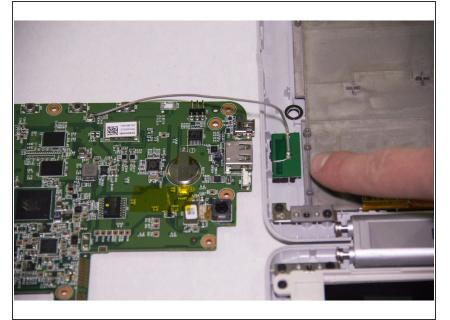
The motherboard is now connected in only one place on the edge of the device. Being careful of this, flip the motherboard outside of the device, leaving it connected to the foam padding inside of the device.
