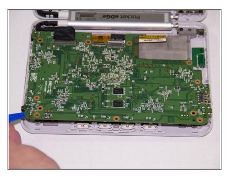
Using the plastic opening tool, carefully pry the bottom of the motherboard up and away from the casing.
