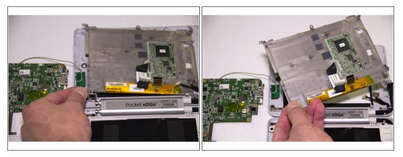
• Carefully pry up the gray plastic e-reader screen using your finger and remove from the device.
