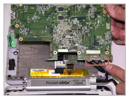
Lift the outer edge of the motherboard up. Carefully disconnect the 3 connections on bottom of the motherboard by pulling gently.
