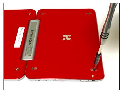
Using your J1 Phillips head screwdriver, remove all eight 6mm screws from the back of your device.
