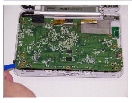
Using the plastic spudger, carefully pry the bottom of the motherboard up and away from the casing.
