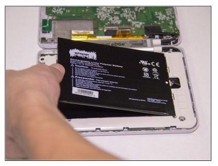
Locate the side containing the battery. Lift the top of the battery out using your finger and the indentation at the top.
