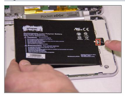
Carefully unplug the bottom side of the battery from the connecting plug and set the disconnected battery aside.
