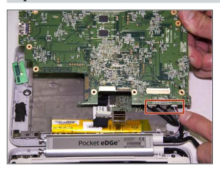
Lift the outer edge of the motherboard up. Carefully disconnect the 3 connections on bottom of the motherboard by pulling gently.
