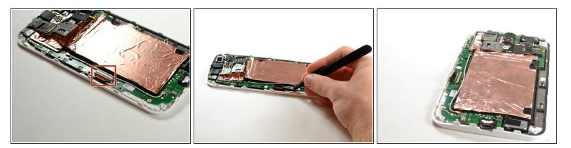
• Remove LCD connector by lifting the black plastic flap.
