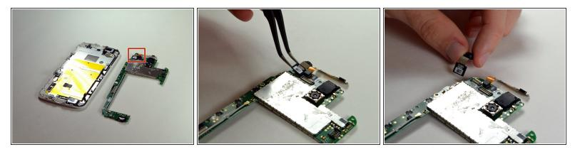
• Use the prying tweezers to remove the front facing camera.
