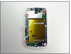
Using a T5 Torx screwdriver, unscrew the three 2.2 mm screws holding the motherboard in place.
