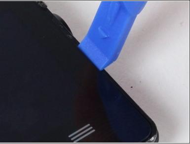
Place the blue plastic opening tool in-between the screen and plastic casing of the watch and slowly pry up one side of the screen.
