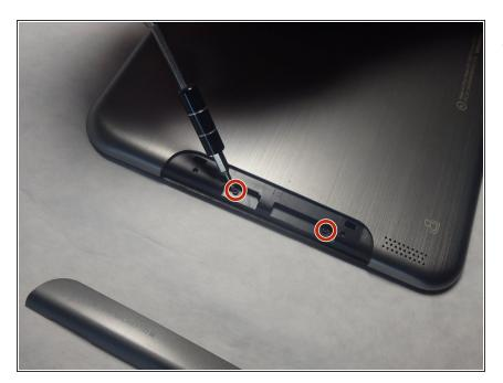
Remove the two 4-mm #0 screws from the inside of the Micro SD compartment.
