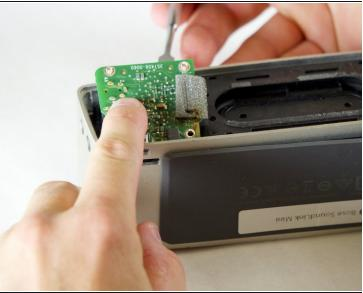
• Remove the circuit board by pushing it with your index finger in the direction shown while using a nylon or metal spudger to lift it up and out of place.
