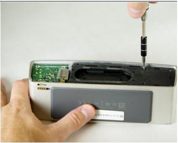
Remove the four 15.0 mm screws on the left and the four 9.0 mm screws on the right using the T8 Torx Screwdriver.
