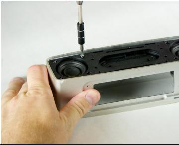
• Remove the eight 9.0 mm screws using the T8 Torx Screwdriver.
