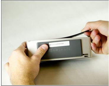
• The grille is attached to the speaker with double sided sticky tape. To remove the grill gently pull upward while keeping tension to the right.
