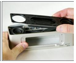
• Using a nylon or metal spudger, pry up the plastic divider and remove it.
