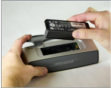
While holding the cover back, pull straight up on the battery to remove it.
