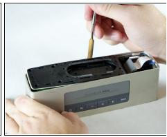
Use a Metal Spudger to pry up the plastic divider.
