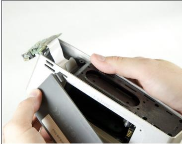
• Carefully pull on the battery cover until the rubber tab slides out of the aluminum casing.
