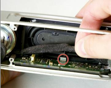
Unhook the speaker wires clipped onto the button switch circuit board.
