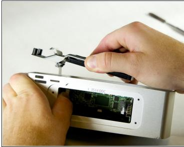
• When removing the plastic divider be careful not to damage the wire strip sliding through it.
