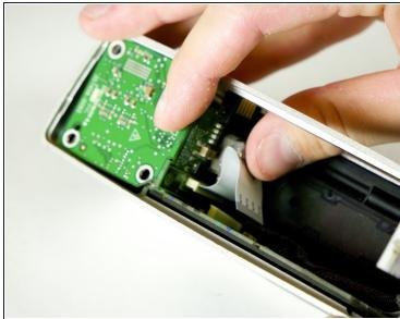
Reach through the battery compartment hole and unplug the power strip shown.
