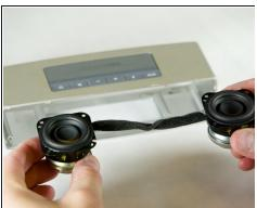
• Gently lift the speakers up and out of the casing.
