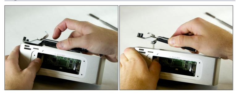
When removing the plastic divider be careful not to damage the wire strip sliding through it.
