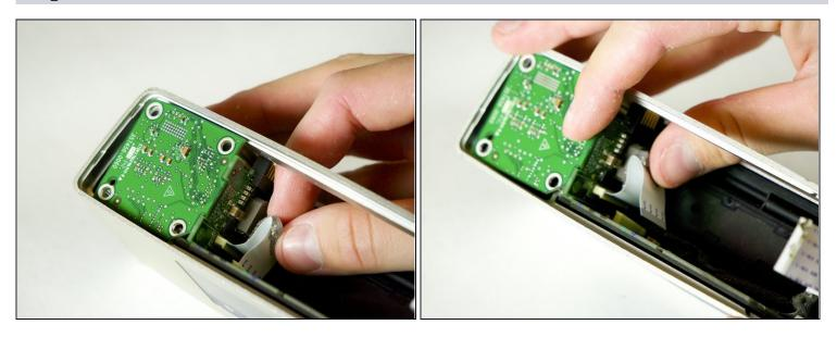
• Reach through the battery compartment hole and unplug the power strip shown.
