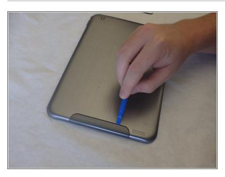
Remove the cover over the Micro SD outlet by using a plastic opening tool to pry open and push out the cover panel.
