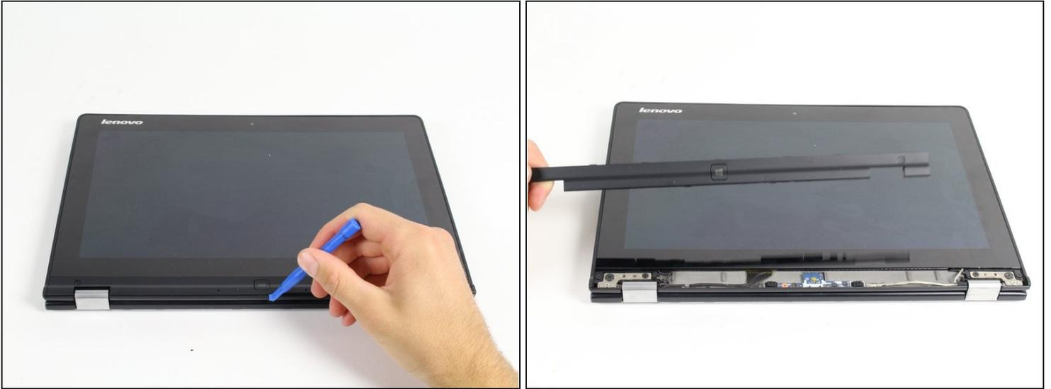
① Flip keyboard under the screen for ease of repair.
