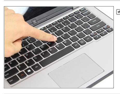
To install a key, apply pressure until it snaps into place.
