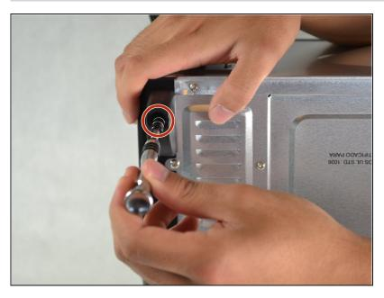
• Remove the 11.5 mm screws using a #2 Phillips screwdriver.
