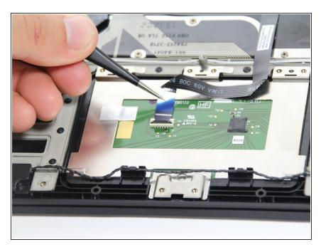
With tweezers, gently slide the ribbon cable out from under the connector.
