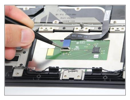
Using a sharp tool such as tweezers, lift up the black cover that is on top of the ribbon cable.
