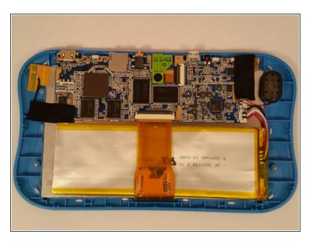
Once opened, carefully peel back the black electric tape around the digitizer.
