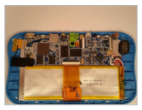
Unscrew the five screws holding down the motherboard.
