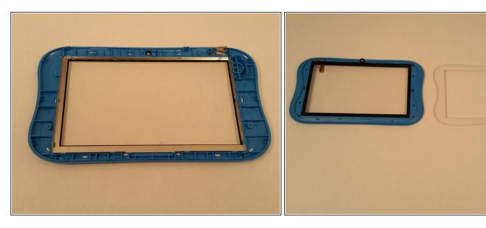
Remove all of the white pegs located along the perimeter of the plastic. You'll need to remove all of the pegs to remove the white front face.
