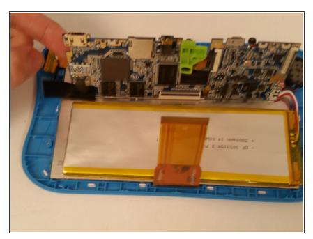
Once all five screws are removed, you should be able to lift up the motherboard.
