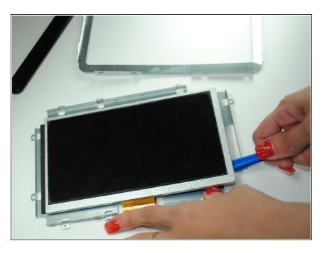
Remove the plastic over the screen and use a spudger or plastic opening tool to remove the screen from the sticky adhesive.
