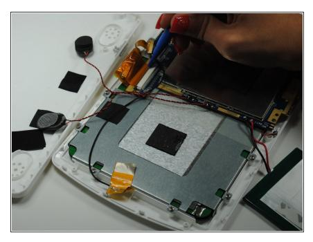
Use a plastic opening tool and place the tip in between the white and black pieces holding in the ribbon cable in to release the three ribbon cables around the motherboard.
