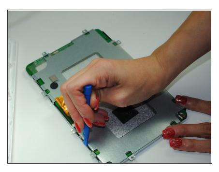
Use a plastic opening tool to undo the metal clips holding the screen in place.
