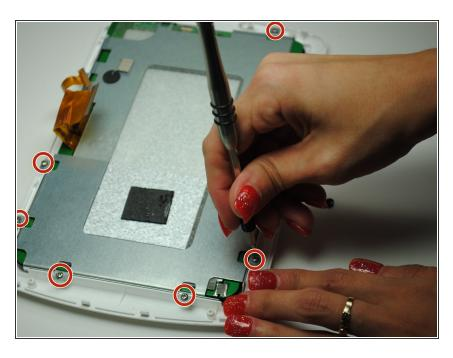
Remove the motherboard and unscrew the twelve 7.0 Phillips #00 screws holding the metal casing around the screen in.
