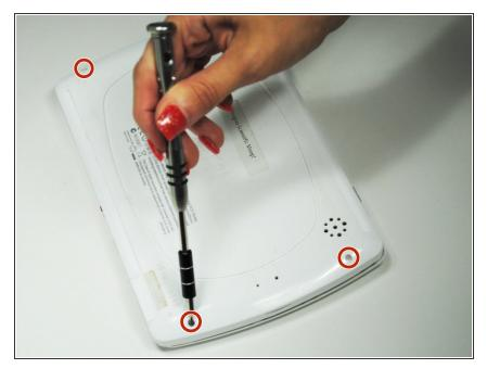
Use a screwdriver to remove the four 7.0 mm Philips #00 screws from the back of the device.
