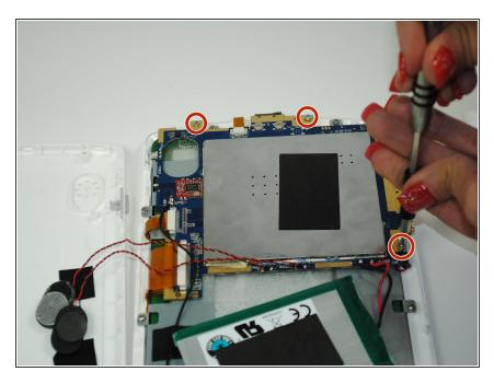
Use a screwdriver to unscrew the three 4.0 mm Philips #00 screws holding the motherboard in place.
