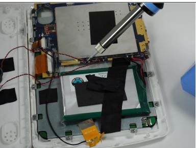
Use a soldering station to disconnect any wires attached to the motherboard.
