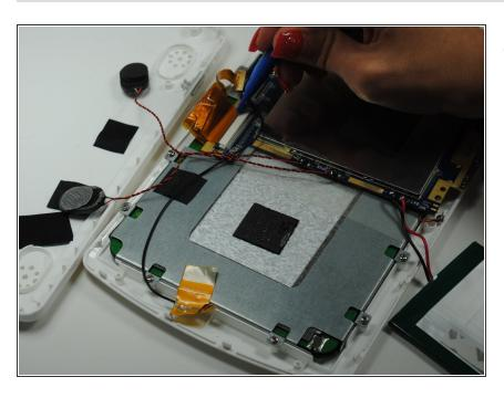
Use a plastic opening tool to release the ribbon cables surrounding the motherboard.
