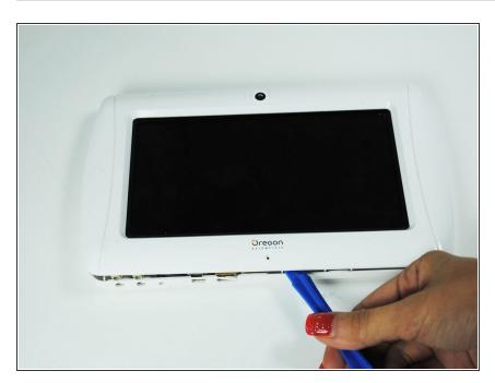
Use a plastic opening tool to detach the clips on the inside of the device.
