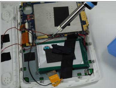
Use a soldering station to separate the wires from the speakers.
