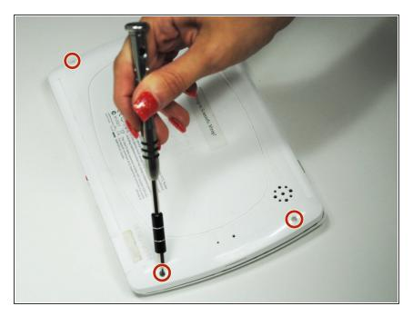
Use a screwdriver to remove the four 7.0 mm Philips #00 screws from the back of the device.
