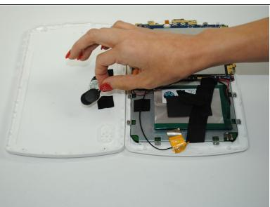
Remove the electric tape holding the wires of the speakers in place and gently pull the speakers out of their slots in the device.
