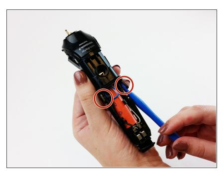
Use the plastic opening tool to separate the clip on the right side of the inner housing.
