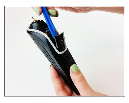
Apply pressure to pry off the power button.
