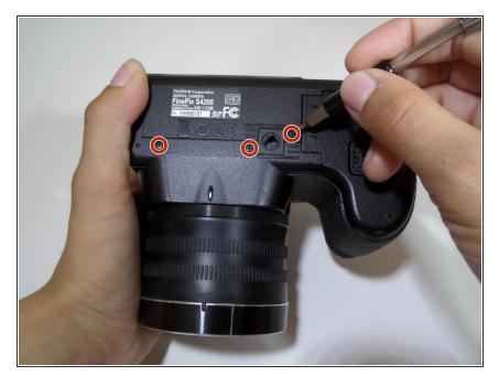
Remove the three 4 mm screws from the bottom of the camera with a Phillips #000 screwdriver.
