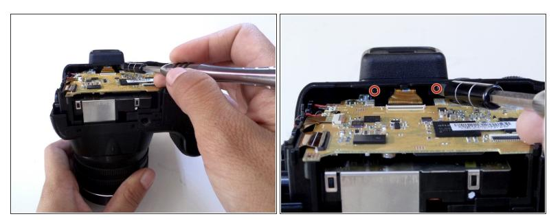
• Remove the two 4 mm screws with a Phillips 000 screwdriver under the viewfinder.
