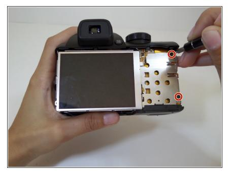
Remove the two 4 mm screws that hold the motherboard and metal plate in place.
