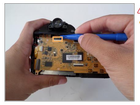
Using the plastic opening tool, pull down the small black latch to remove the orange ribbon from the mother board.
