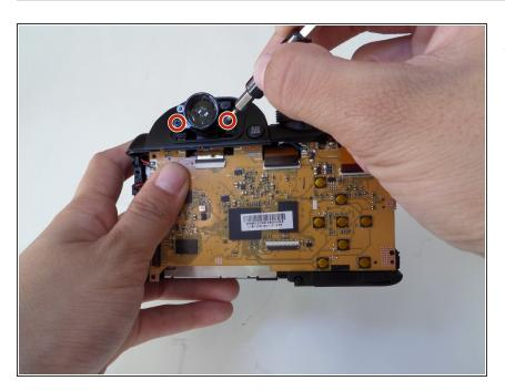
Remove the two 3mm screws surrounding the viewfinder with a Phillips 000 screwdriver.
