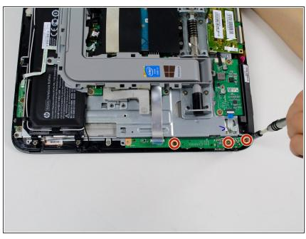
Remove the three 6.35 mm PH#0 screws around the USB board.
