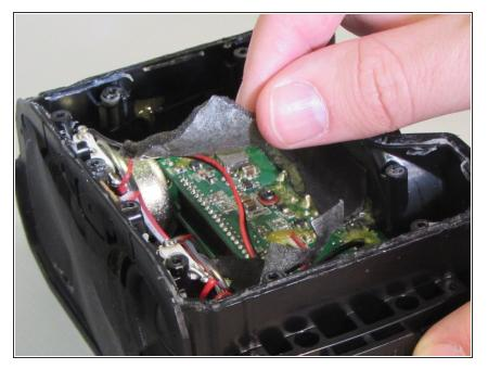
• Remove the foam padding located in the Braven BRV-1s.
