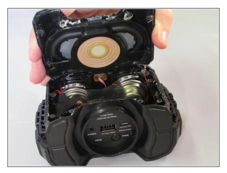
• Pull upward on the woofer until it is removed.
