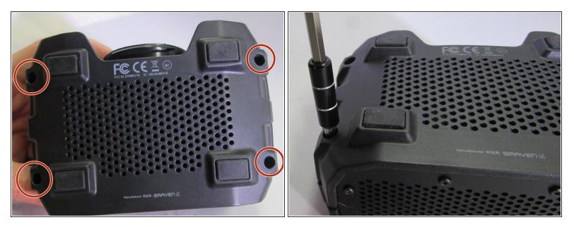
Using a 0mm Philips Head screwdriver, unscrew the four 0.9mm screws located on the bottom of your device.
