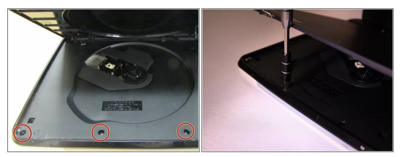
Open the disc flap and remove the screws inside with the Phillips #0 screwdriver. There will be three screws.
