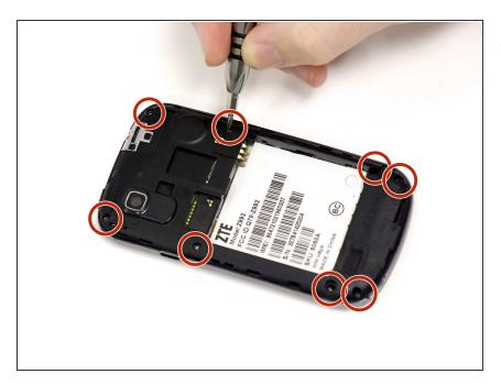
Using your J00 screwdriver, unscrew each of the 8 Philips head screws from the black plate of the device.
