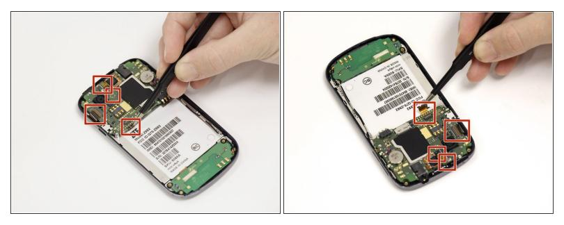
Using the tweezers remove the 4 orange ribbon cables. Do this by lifting their corresponding black connectors and pulling the ribbon out.
