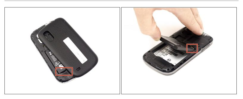
• Remove the battery by the notch in the back plate.
