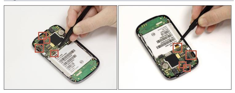
• Using the <u>tweezers</u> remove the 4 orange ribbon cables. Do this by lifting their corresponding black connectors and pulling the ribbon out.
