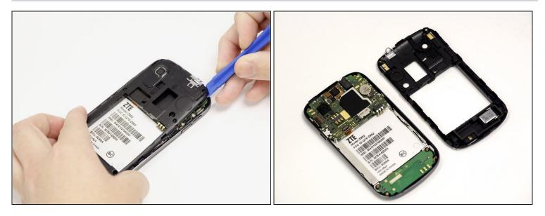
• Using the spudger tool, pull up from underneath the back plate and pop off the piece.
