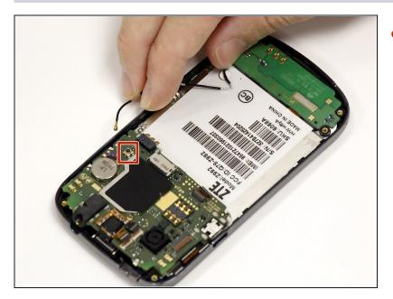
• On the left side you will see a cellular antenna cable wire. Remove this wire by gently pulling it off.
