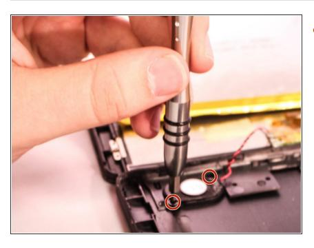
Using a Phillips #000 screwdriver, remove the two 3.0mm long screws shown in the illustration.
