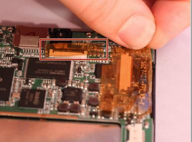
• Locate the three ribbon cables connecting components to the motherboard. The connections are covered with orange shielding tape. Peel the tape off the connectors and reserve for reassembly.
