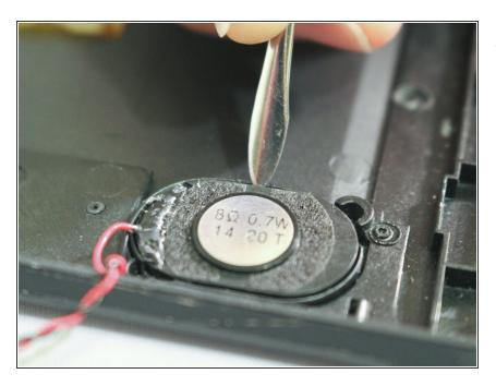
Using the spudger, gently pry the speaker from it's plastic socket.
