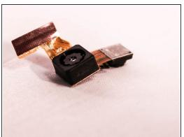
• Insert the flat end of the spudger into the groove between the external camera and the tablet's plastic case. Then, applying a gentle prying motion on both sides of the camera, loosen the glue holding down the external camera to separate it from the plastic case.
