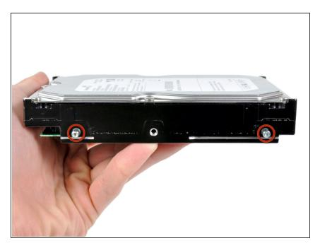
Remove the two T8 Torx retaining posts from the other side of the hard drive.
