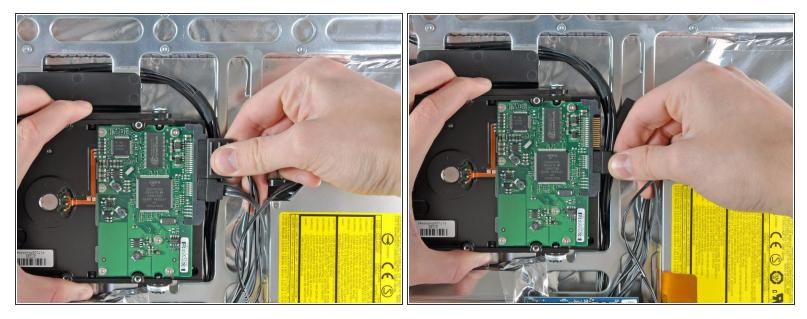
• Disconnect the SATA data and power cables by pulling their connectors away from the hard drive.
