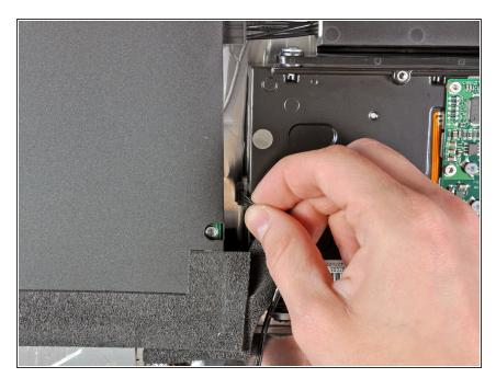
Disconnect the hard drive thermal sensor cable from the thermal sensor attached to the side of the hard drive.
