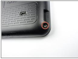
Remove the four 9mm screws on the back of the GPS unit with the T4 mini screwdriver found in the iFixit Pro Tech Tool Kit.
