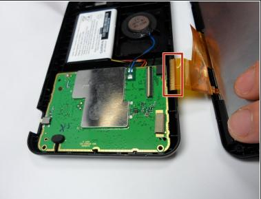
After the GPS unit is open, gently separate the orange ribbon cord connecting the LCD to the motherboard. Separate the cord at the motherboard.
