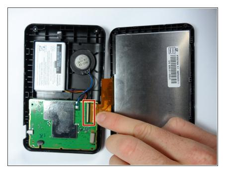
Using the replacement LCD screen, plug the orange ribbon cord into the motherboard.
