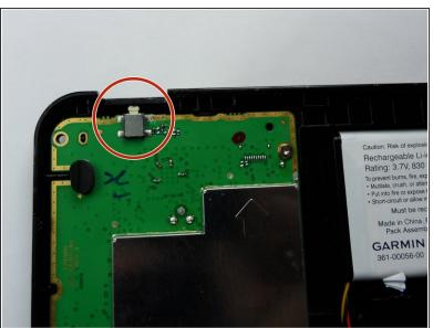
• Look for a small button on the motherboard at the top of the device, and insert replacement power button on top of the small button on the motherboard until you hear a click.
