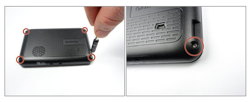
• Use the T-4 screwdriver to unscrew the 9 mm screws on the back of the device.
