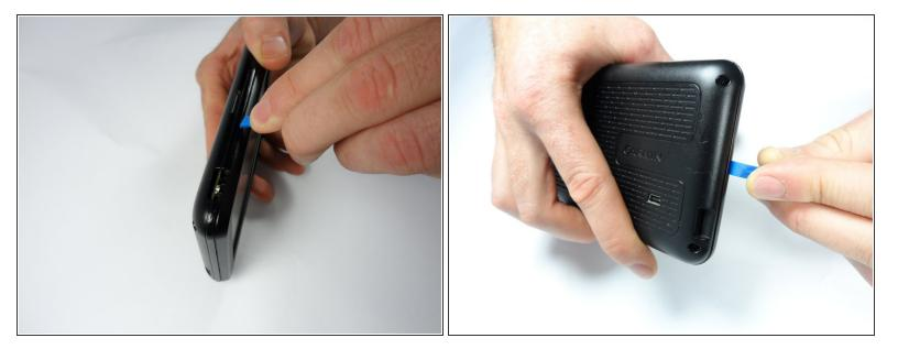
Pry open the device from all four sides using the iFixit Plastic Opening Tool until you see the inside of the system.
