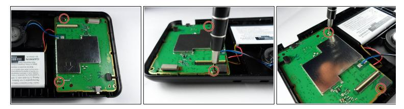
• After the GPS is open, remove the two 9 mm screws holding the motherboard in place.
