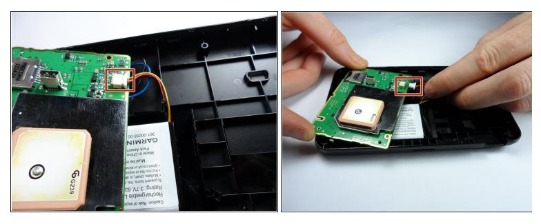
• Unplug the red and yellow cables from the motherboard to remove the battery.
