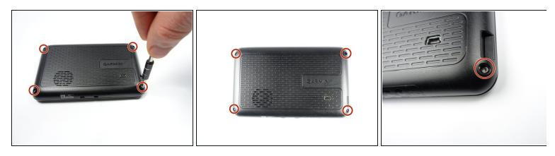
• Remove the four 9 mm screws on the back of the GPS with the T4 Torx screwdriver.
