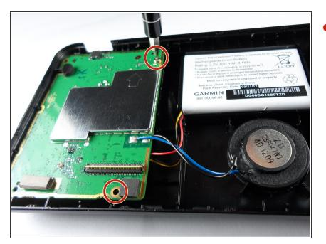
Remove the two 0.5 cm screws using the T4 Torx screwdriver attaching the motherboard to rear cover of the GPS unit.
