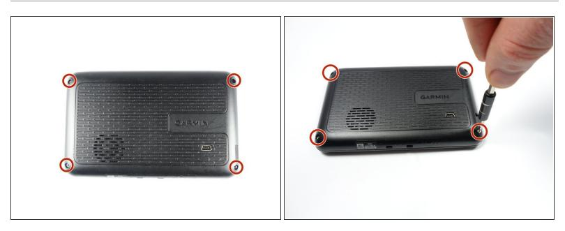
• Remove the four 9 mm screws on the back of the GPS with the Torx T-4 screwdriver set.
