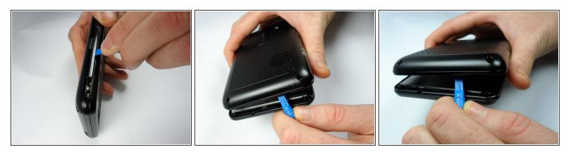
• Use the iFixit Plastic Opening Tool to separate the front cover and the rear cover on all four sides.
