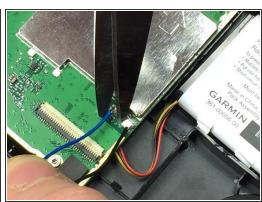
Cut both wires using a pair of wire cutters.
