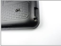
Remove the four 9 mm screws on the back of the GPS unit using the Torx T-4 screwdriver found in the iFixit Pro Tech Tool Kit.
