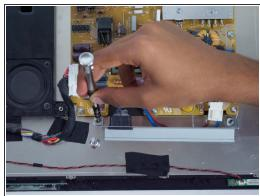
With the Phillips #02 screwdriver, remove the two 5mm length x 7mm head screws from the left and right side of the power port plate.
