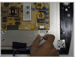
Remove the power port by depressing the white tab attached to the wires.
