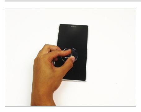
Once the screen is heated sufficiently, press the small suction cup to the center of the screen.
