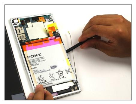
Insert the spudger underneath the battery and run it back and forth to remove any adhesive.
