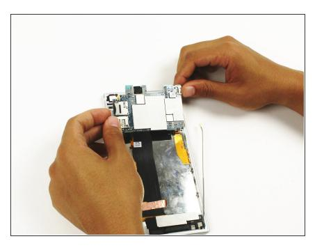
Detach the upper end of the motherboard by pulling the top end upwards.
