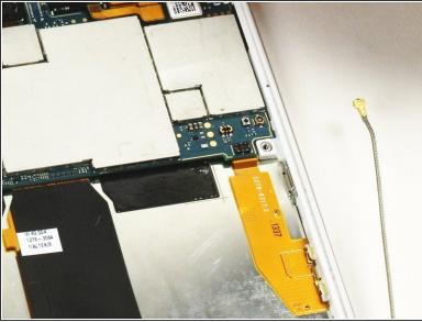
Disconnect the ribbon cable at the bottom right of the motherboard. (It's shown tucked under the motherboard in this photo, which is incorrect—don't do this!)
