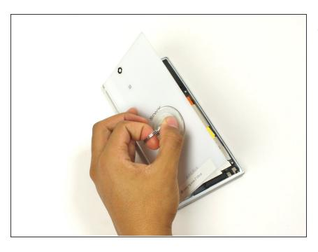
Remove the back panel by pulling the small suction cup upwards.
