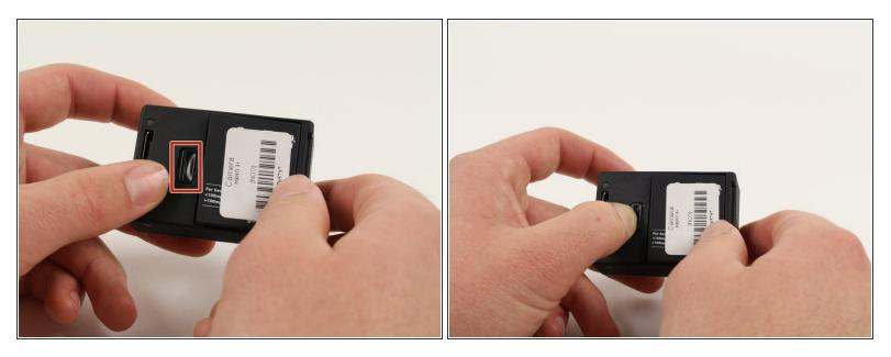
• Push the tab on the back of the device left to remove the plate covering the battery.
