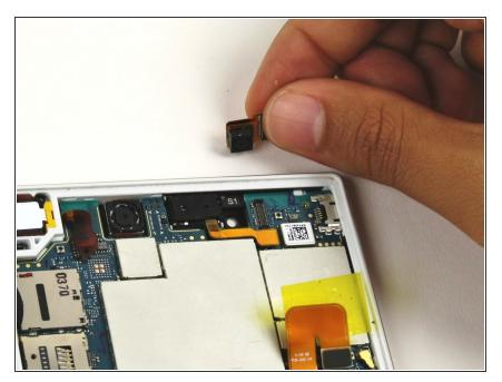
• Remove the front facing camera by pulling upward on the flap to its right
