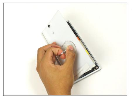
• Remove the back panel by pulling the small suction cup upwards.
