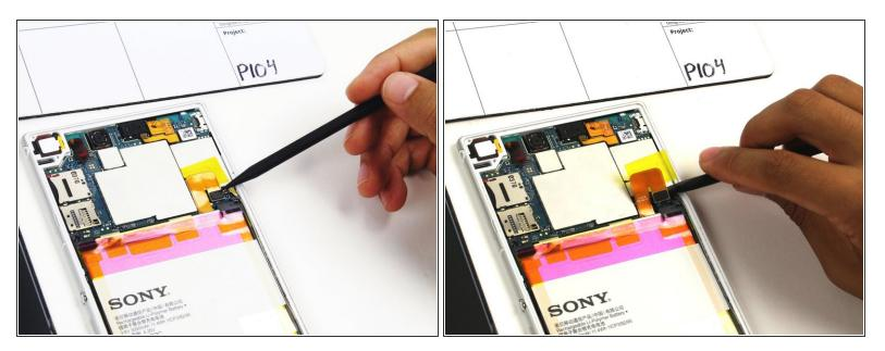
• Detach the battery connection cable by prying it upward with the spudger.
