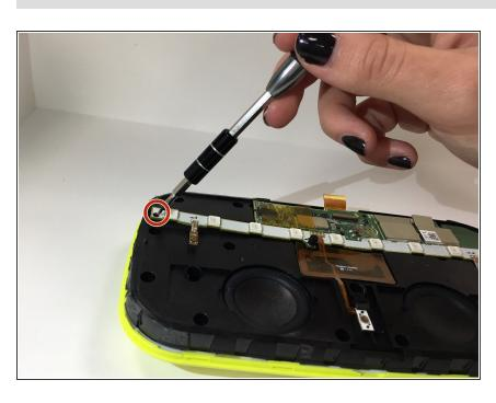
Using a PH00 screwbit, unscrew the two three-tenth screws that hold down the LED light strip at both ends.
