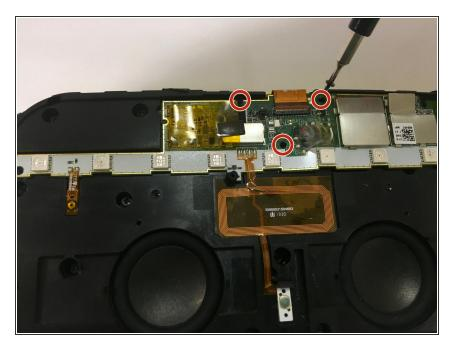
Using a PH00 screw bit, unscrew the three screws that hold down the motherboard.
