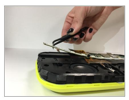
Once unscrewed, the LED light requiring repair can be accessed by lifting up the entire LED light strip with tweezers.
