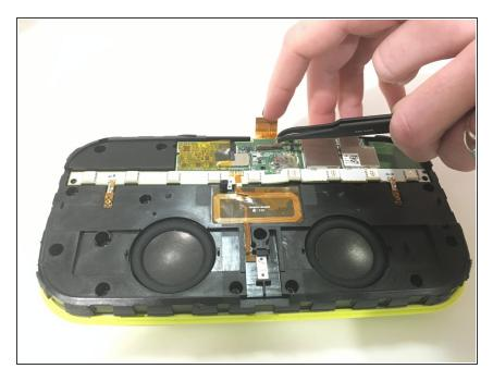
Use tweezers and fingers to lift tab and ZIF (zero insertion force) connecter.
