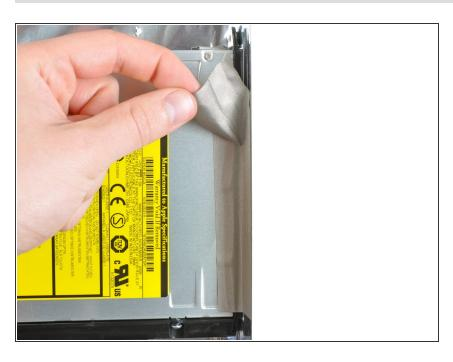
Peel off the strip of EMI tape attaching the right side of the optical drive to the rear case.
