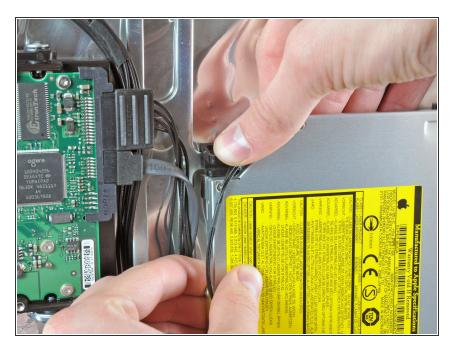
Push down on the optical drive bracket retaining clip while pulling the top edge of the optical drive away from the rear case.
