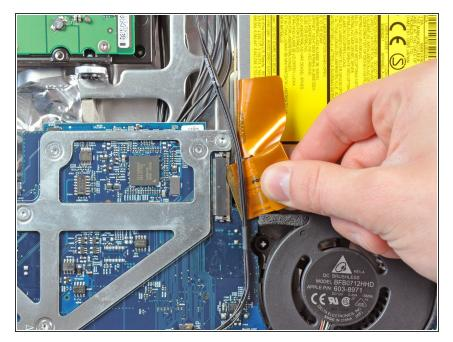
Pull the optical drive ribbon cable out of its socket, being careful not to rip it in the process.
